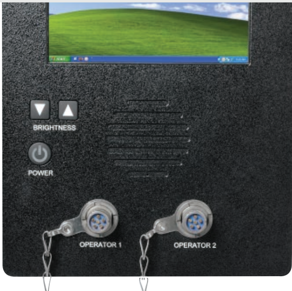
Two external headsets can be connector through ports on the front of the DRAP.
