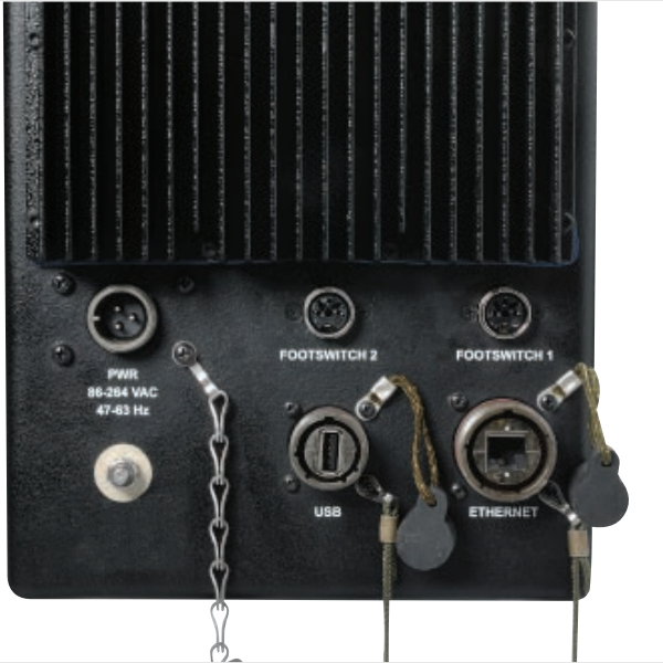
USB, Ethernet, Power and operator footswitch connectors are located on the rear of the unit below the passive heatsink.
